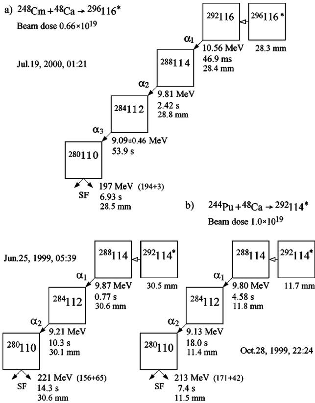
FIG. 1. (a) Time sequence in the observed decay chain. (b) Two decay sequences of  $^{288}_{114}$  observed in the  $^{244}\text{Pu} + ^{48}\text{Ca}$  reaction. Vertical positions of the observed events are given with respect to the top of the strip. Values in parentheses show fission energies measured by the focal-plane and side detectors, respectively.
